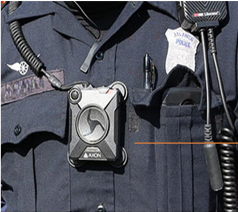
Body worn camera attaches to uniform with magnetic clip
